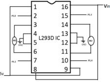
Fig. 4. Circuit diagram of Motor Driver interfacing Arduino
