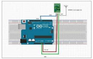
Fig. 3. Circuit diagram of RF jammer
