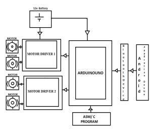
FIG. 1.BLOCK DIAGRAM OF PROPOSED ROBOT
